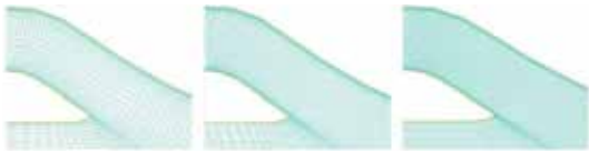
Fig. 4 Grid topology of mid-longitudinal section
